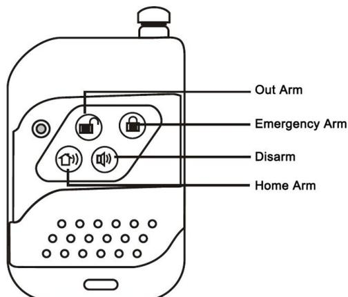
The remote controller has 4 keys: **Disarm**, **Out Arm**, **Home Arm** and **Emergency Arm**.
