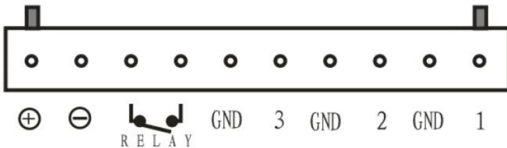
The first and second ports (⊕ ⊖) are internal power source output pin (load capacity: 12V/300mA output).
